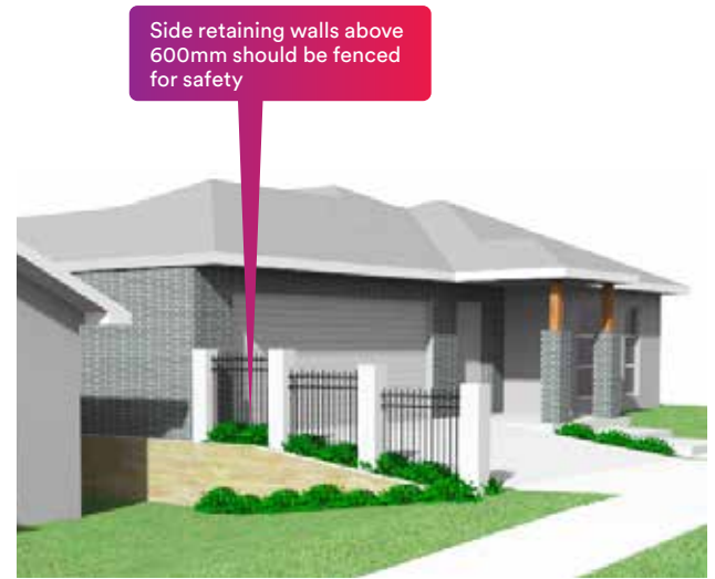
Retaining walls forward of the home must taper on side boundaries
