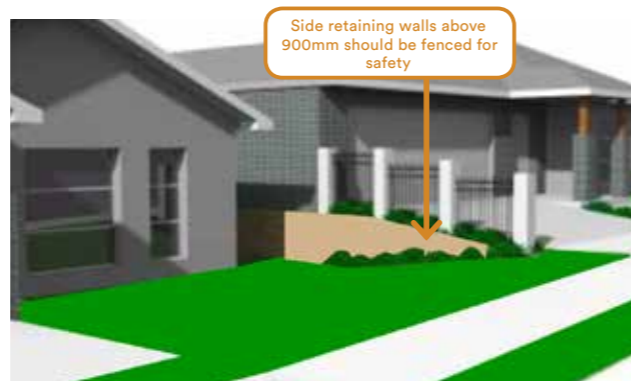
Retaining walls forward of the house
