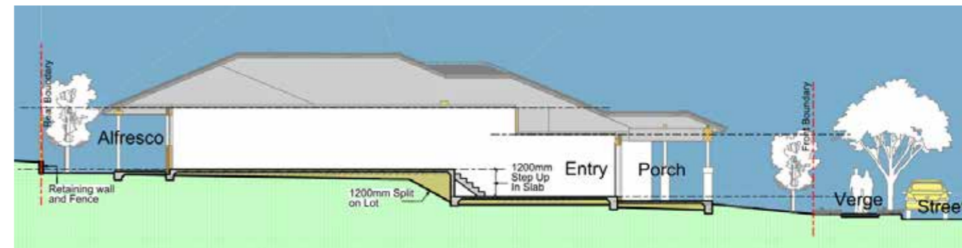
1.2 metre split - step up from front boundary
