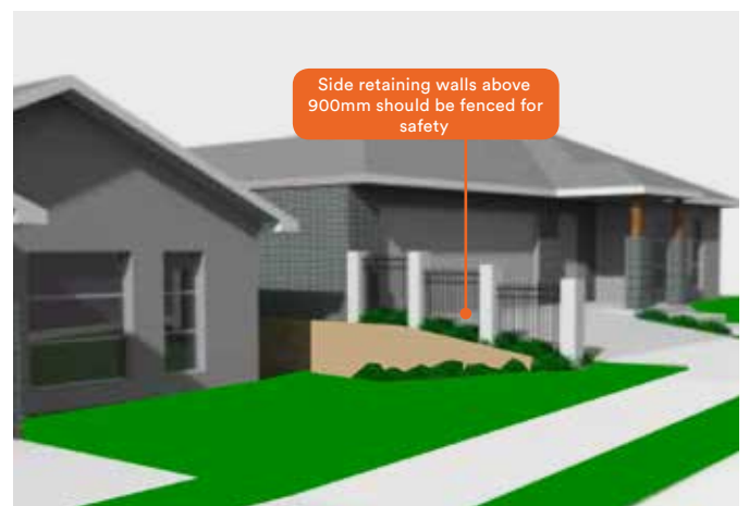
Retaining walls forward of the house
