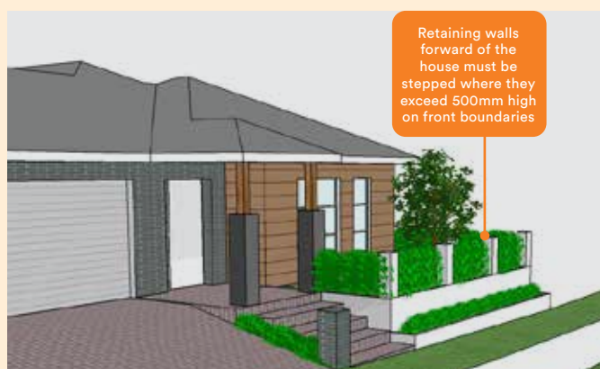
Retaining walls forward of the house
